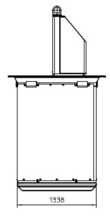
Figure 1: Details of 3cu.m. unit Fully Underground Bin
