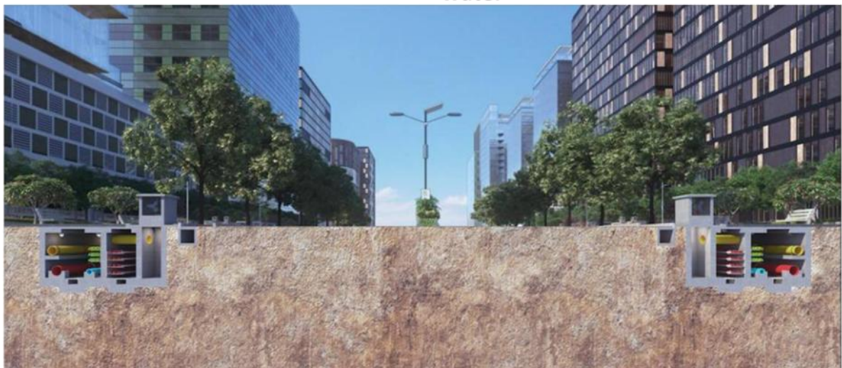
Utility Duct for Infra-Services
